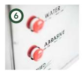
Pneumatic switches provide easy activation of metering valve & water pump.
