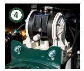
Pneumatic double-diaphragm water pump.
