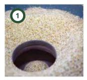
Concave top for rapid filling of pot is sealed automatically by a heavy duty pop-up valve.
