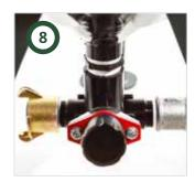
Fitted with abrasive control valve with Tungsten adjusting bar.
