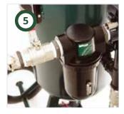
Moisture water separator. Assists in removing the water and moisture from the incoming compressed air supply to the blast pot, helping to ensure that the abrasive does not become damp.
