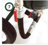
Flexible pusher line guarantees air flow without pressure loss caused by elbows, and eases valve replacement.
