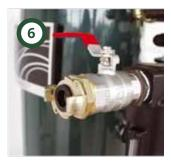
Quick Claw coupling for quickly attaching air supply hose.
