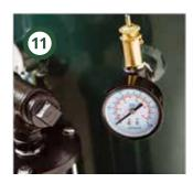
Pressure gauge and pressure relief valve.
