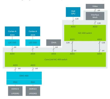
The previous diagram shows all the connections where AXI is used. You can see that AXI3 and AXI4 are used within the same SoC, which is common practice. In such cases, the interconnect performs the protocol conversion between the different AXI interfaces.
