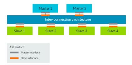
An Arm processor is an example of a master, and a simple example of a slave is a memory controller.
