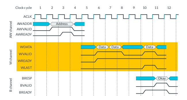
In this case, the AW channel indicates a sequence of three transfers, and on the W channel, we see three data transfers.
