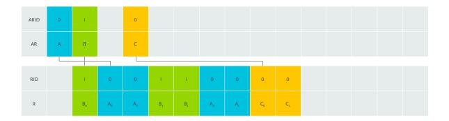
Because transaction A was requested before transaction C, the slave must return all four R data values for A before the data values for C.
