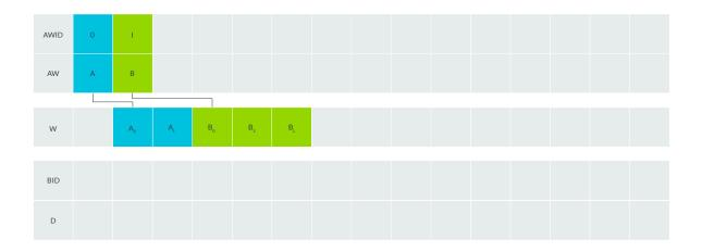
In this example, the master issues address A then B, so data must start with AO before BO.
