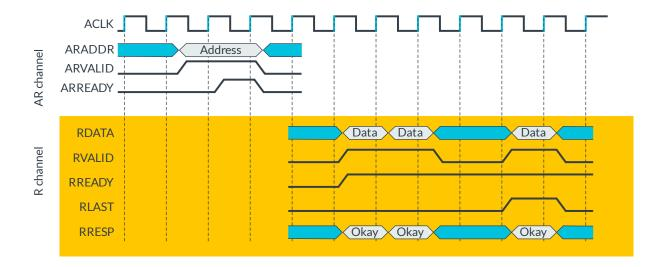
In this example, we transfer a single address on the AR channel to transfer multiple data items, with associated burst width and length information.
