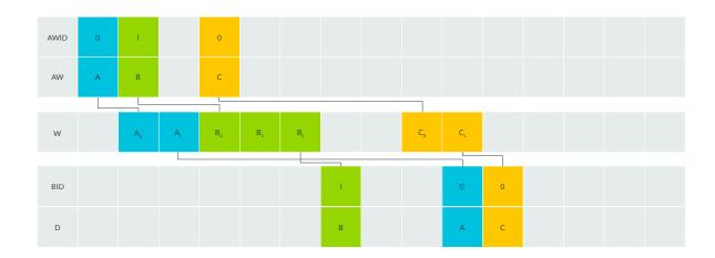
In this example, transaction B has a different ID from the other transactions, so it can complete at any point. However, transactions A and C have the same ID, so they must complete in the same order as they were issued: A first, then C.
