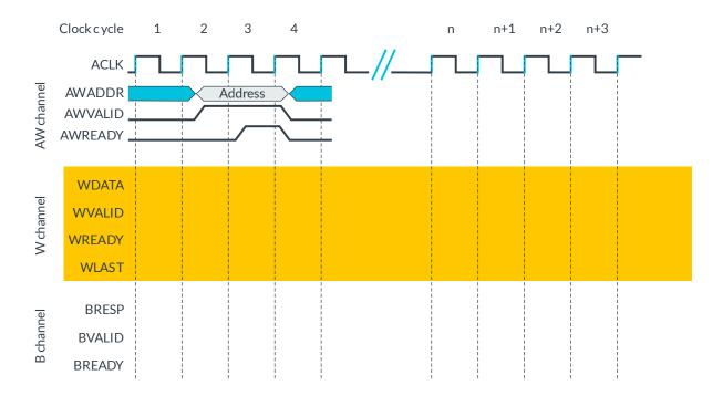
This handshake is where the master communicates the address of the write to the slave. The handshake has the following sequence of events:
