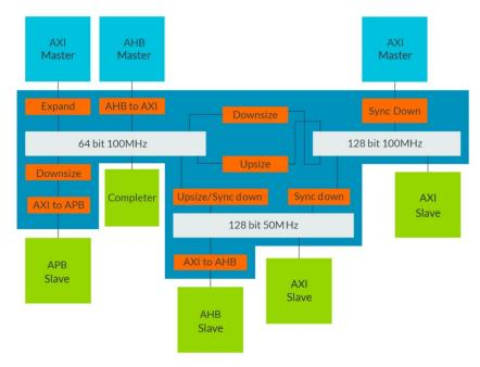
The following diagram shows an example of an SoC with various processors and function blocks:
