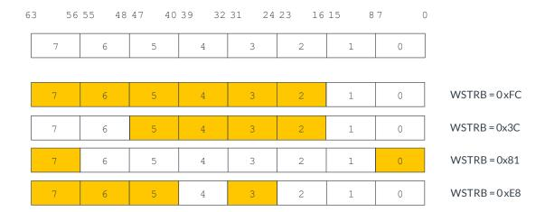
Looking at the first example, we suppose that the valid data are only in the top six significant bytes of the data bus, from byte 7 to byte 2. This means that the master has to control the **WSTRB** signal with the hexadecimal value 0xFC.
