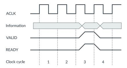
Again, the handshake completes on the rising edge of clock cycle 4, when both **VALID** and **READY** are asserted.
