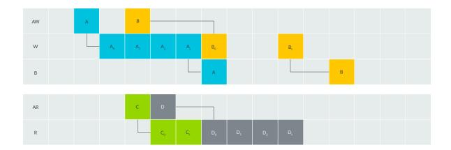
In this example, the master starts transaction B before it has finished transaction A.
