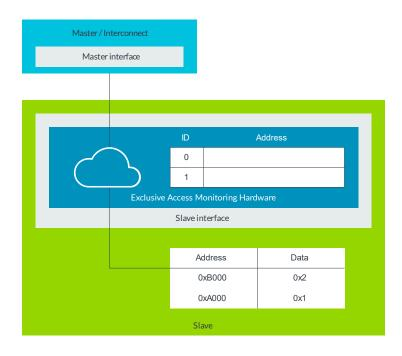
The slave interface includes exclusive access monitoring hardware that can save the ID and the address accessed for each transaction.
