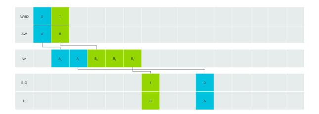
In this example, transaction B completes before transaction A, even though transaction A started first.
