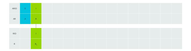
• The read data for the different IDs on the R channel can be interleaved, with the RID value differentiating which transaction the data relates to.
