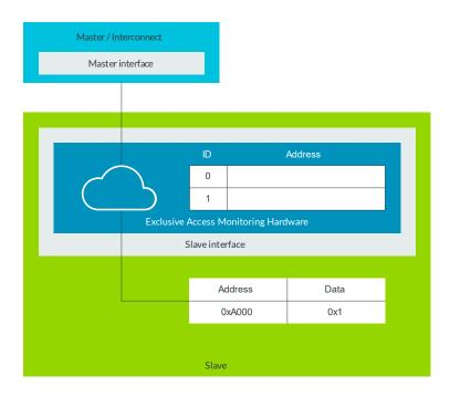
The slave interface includes exclusive access monitoring hardware that can save the ID and the address accessed for each transaction.
