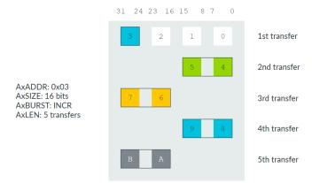
If the transaction were aligned to a start address of  $0 \times 00$ , the result would be a five-beat burst with a width of two bytes giving a maximum data transfer of 10 bytes. In this example, the first transfer starts at an unaligned address of  $0 \times 03$  and contains one byte. All the following transfers in the burst are aligned with the bus width and are composed of two bytes each.
