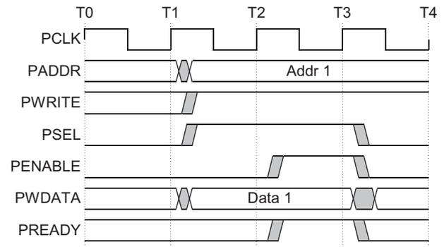
**Figure 3-1 Write transfer with no wait states**
