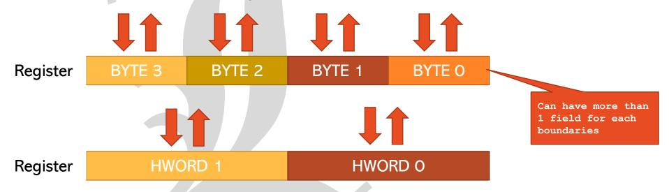
• It supports all IEEE field access types, while systematically verify the byte accesses, hword accesses of DUT.
