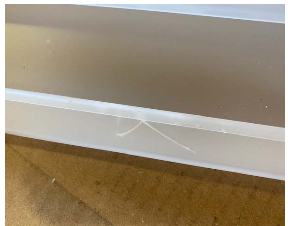
A crack on the other strip light lens
