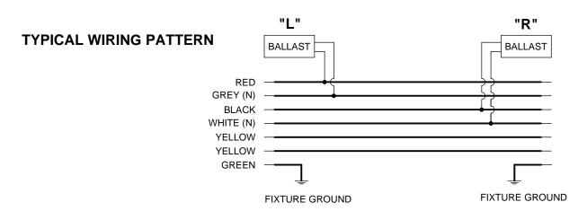
YELLOW WIRES FOR 3-WAY SWITCHING INCLUDED ON "2Y" FIXTURES ONLY
