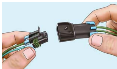
Through wiring with quick connect options
