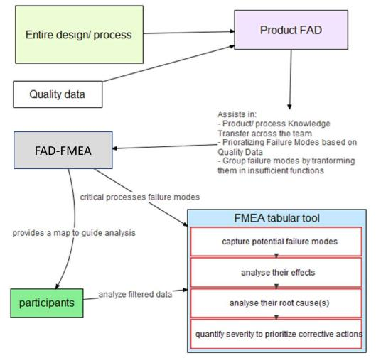
FAD-FMEA was developed to optimise the recourse-efficiency of the FMEA process, and in particular, its initial phase
