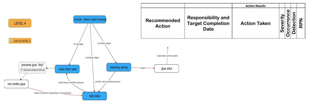
\* There is no universally accepted threshold for RPN. However, values above 100 or the highest three are normally actioned
