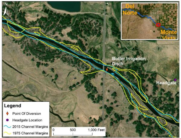
Map showing Butler Irrigation Ditch diversion dam and headgate location. Also shown are 1975 and 2015 Rio Grande channel margins.
