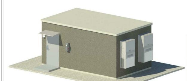
**DESIGN SPECIFICATIONS Building Model:** RCS - 1220 20'-0" Long x 12'-0" Wide x 10'-2" Tall **Building Dimensions:** 19'-0" Long x 11'-0" Wide x 9'-2" Tall Finished Interior Dimensions: Weight: 57,000 lbs. Floor Loading: 250 PSF Roof Loading: 65 PSF 150 MPH Wind Speed: Floor Thickness: 6" Thick Roof Thickness: 4-1/2" Thick 5000 psi Lightweight Aggregate Concrete: Fire Rating: Low seismic, <50%G seismic acceleration Seismic: Level IV: 30-06 Fired from 15' Bullet Resistance: Electrical: 200A
