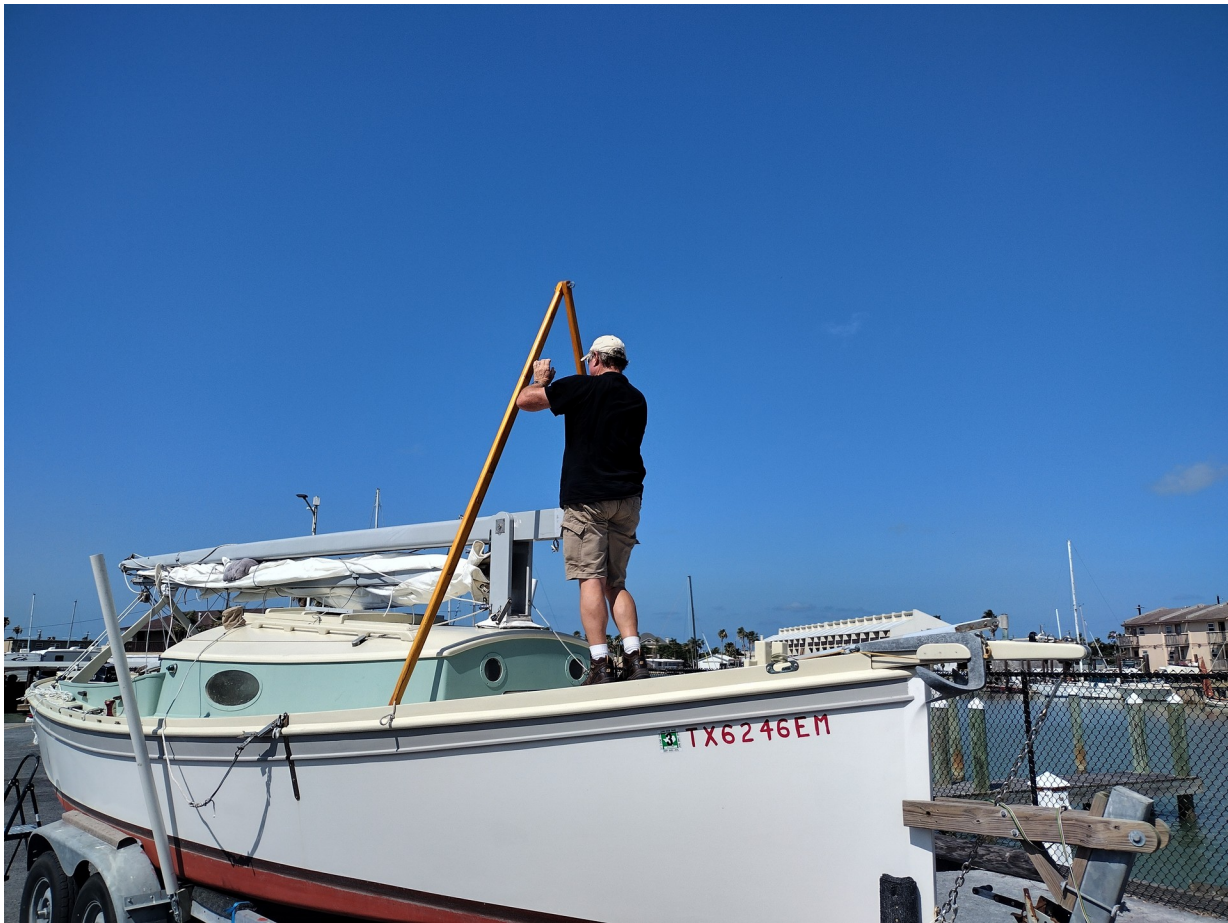
Figure 1: Buddy Simons prepping the gin pole for stepping the mast.
