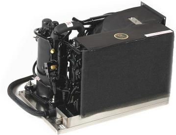
Dimensions: L-23", W-17", H-16.75" Left and Top discharge, add 1" in length Weight : 92 Lbs Amp: 10.4 Cool (220v) 11.4 Rev/Cycle Heat (220v) Blower CFM: 820 Cooling Capacity: 2,400 Cubic ft. Designed to cool 40' cruiser or a 45' sailboats and up (Right Discharge Shown Above) Electric heat not available
