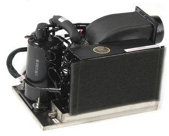
Dimensions: L-16", W-11.5", H-11.5" (Left and Top discharge, add 1" in length) Weight : 48 Lbs Amp: 7 Cool, 8 Rev/Cycle Heat Electric Heat is 18.5 amps @ 115V \*\***Available in 110V OR 220V**  Blower CFM: 320 Cooling Capacity: 800 Cubic Ft. Designed to cool up to a 30' cruiser or a 32' sailboat. (Right Discharge Shown Above)
