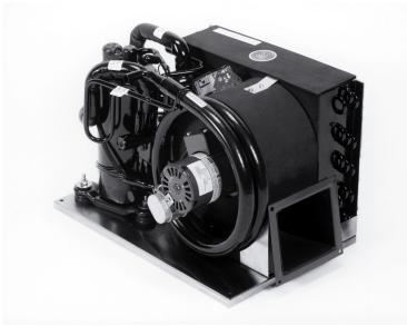
Dimensions: L-19.75", W-13.5", H-13.75" (Left and Top discharge, add 1" in length) Weight : 68 Lbs Amp: 12 Cool, 13.5 Rev/Cycle Heat \*\*Available in 110V OR 220V Blower CFM: 485
