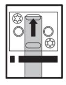
Heating cable inner jacket visible in top window
