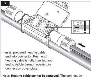
and end seal are designed to be installed only once; the
