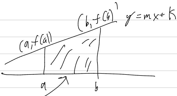
$$\text{Area} = \text{Average height} \times \text{width} = \frac{f(a) + f(b)}{2}(b-a)$$
