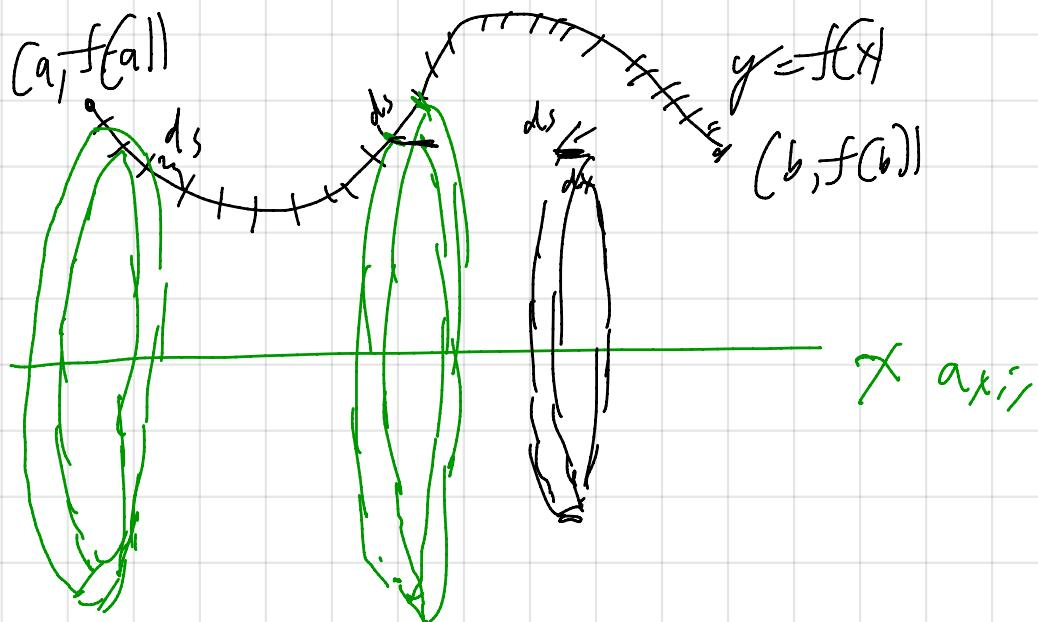
We divide our curve into many tiny pieces, each of length  $ds$ . We then rotate each tiny piece about the  $x$  axis to get a "slanted ring".
