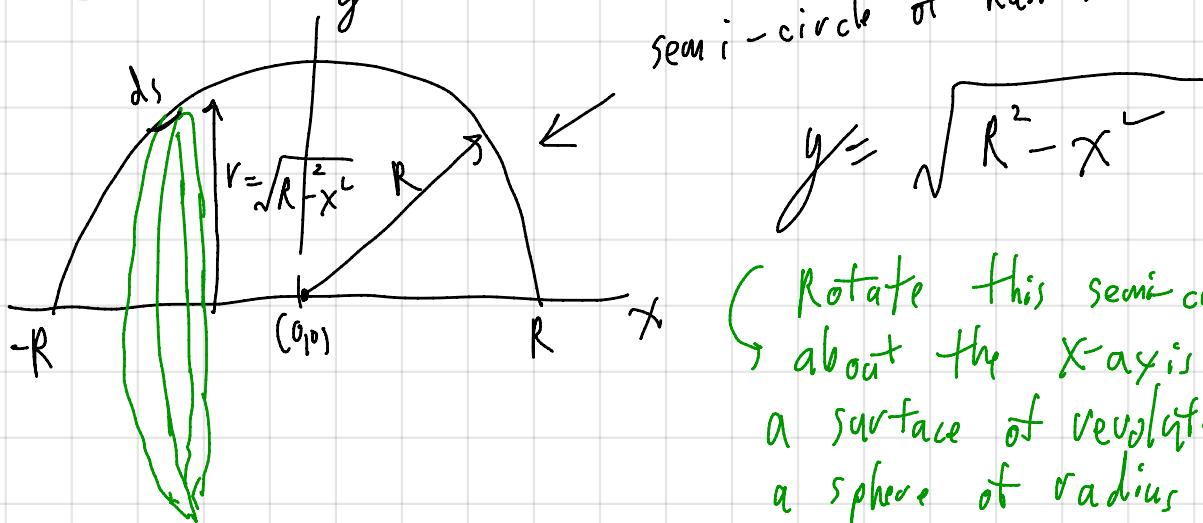
$$2\pi \int_{-R}^R r \, ds = 2\pi \int_{-R}^R \sqrt{R^2 - x^2} \sqrt{1 + \left(\frac{dy}{dx}\right)^2} \, dx$$
