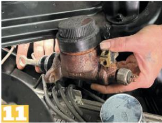
11. One of the things our car owner wanted to change in the brake system was the master cylinder — like most cars of the period, this Comet used a single-circuit master. These work fine when everything is in order; however, if a leak develops anywhere in the system, before long, the driver will find zero braking available. Our disc-brake kit included a dual-circuit master from a later Ford application.
