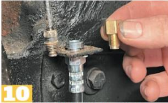
10. Our conversion kit was intended for a few different Ford applications, so it included some fittings and such that we did not need. Among them were these hardline adapter fittings, which would merge the disc-brake flex hoses with the hardlines on some drum-brake cars. For this Comet, the hardlines connected directly to the new flex hoses.
