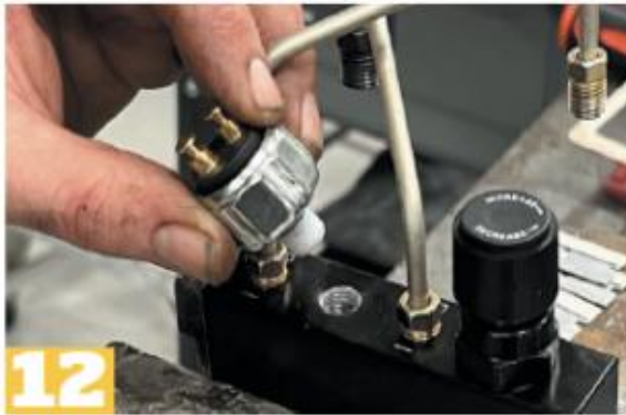
12. We were pleasantly surprised to find that our stock-style disc-brake kit included an adjustable proportioning valve. This one will mount neatly right underneath the master, but before putting it on, we needed to mount the pressure switch that activates the brake lights, which was also included.
