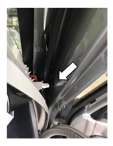
6. POWER & EARTH SELECTION Pictured are the fused terminals that provide the easiest power supply for the console. The wires can be brought up through the bottom of the power box and be connected to the (–neg) Earth terminal. You can choose to connect to constant power – 12V battery (BATT) or accessory power – 12V accessory (ACC). i.e. on with the key.
