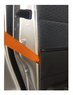
GXL MAP POCKET REMOVAL Remove the 5 screws holding the map pocket to the card of the door and discard the screws.
