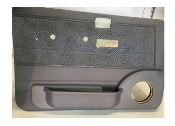
9. MARKING SPEAKER HOLE While the pod is in place; trace around the inside of the speaker cut out.
