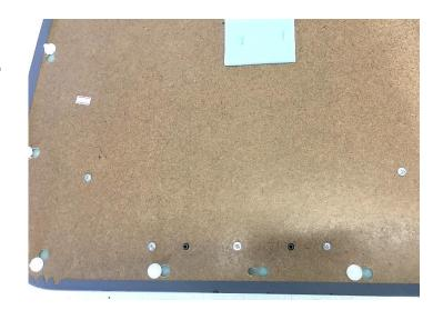
6. MAP POCKET ATTACHMENT Using 5 of the new screws supplied, attach the factory Toyota map pockets to the new speaker pods. The 2 large dowel holes will help locate the screw holes; make sure that the screws are not over tightened.
