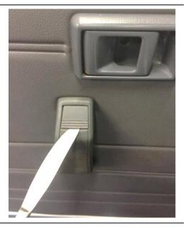
3. WORKMATE & GX – Card Removal Slip a rag between the window winder and the clear plastic washer while the handle is facing up. Pull the rag from side to side; the rag will grab the end of the circlip and it will pop off the handle. Push the circlip back into the handle; this way the winder can be pushed back into the spline upon door re – assembly.
