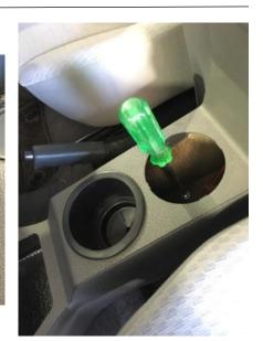
Tip: at this stage do not tighten the cup holder screw.
