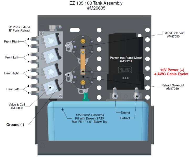
Central tank assembly is typically located near the "center" of the unit, Example: In front of rear axle on driver side frame rail (outside or between rails). Can be mounted to existing boxes, sub-frame, etc.
