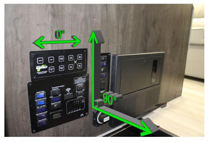
\*Control panel cannot be mounted on an angled surface or tethered.
