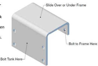
strong enough to support the weight of the assembly (7/16" hardware and lockwasher required, torque to 70 ft/lbs.).
