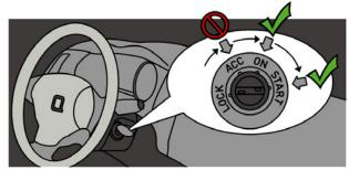
Turn vehicle ignition to the ON/RUN or START position.
