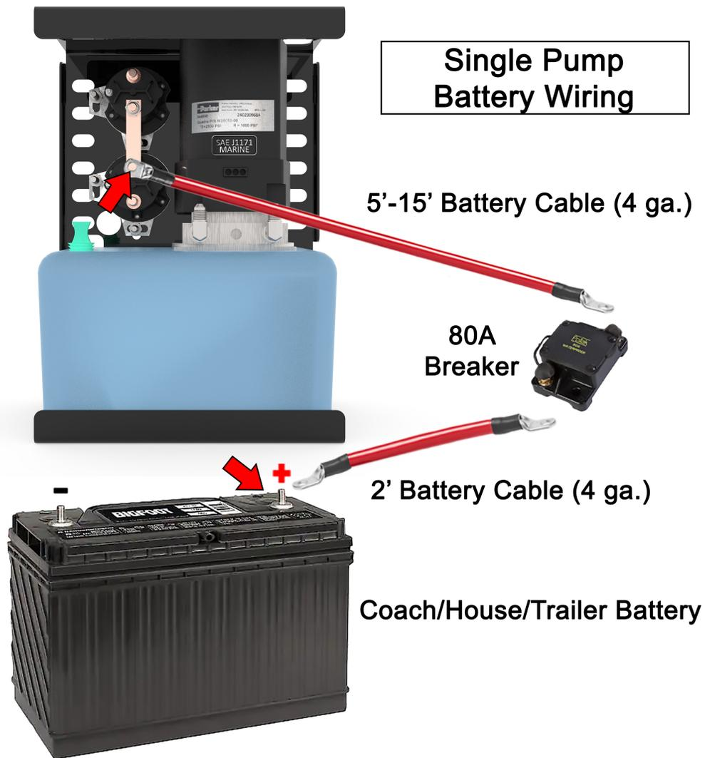
The hydraulic system requires 12 volt battery - use at least a 4 gauge battery cable for the power.
