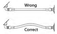
6. Protect hydraulic lines from damage, keep away from heat and moving parts (exhaust, suspension, driveshaft, etc.) and from sharp edges that could cut/damage the line when making contact while operating or driving.
