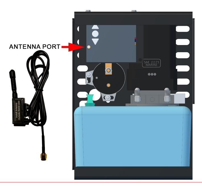
**ATTENTION**: Antenna must be installed in a location outside of the pump assembly.
