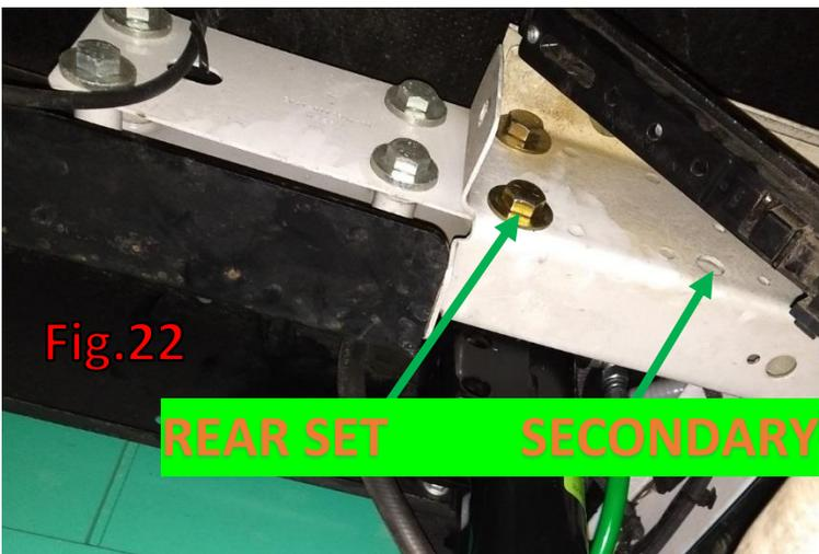
LOCATE FRAME EXTENSION LOCATION ABOUT 3-4FT BEHIND REAR AXLE, JUST REAR OF THE REAR LEAF SPRING MOUNT (Fig.26). CYLINDERS CAN UTILIZE EXISTING HOLES IN THE FRAME, AND CAN BE MOUNTED ON THE OUTSIDE OR INSIDE FACE OF THE FRAME, OR ONE OR THE OTHER. THERE ARE TWO SETS OF HOLES TO LOOK FOR ON THE FRAME NEAR THE FRAME EXTENSION:
