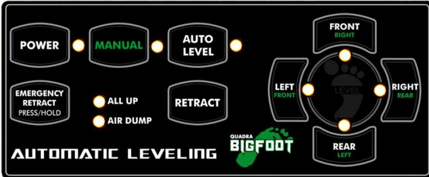
**ALL LIGHTS ARE FLASHING, THIS MEANS PANEL IN ZERO OR PROGRAMMING MODE, SEE NEXT PAGES. SOME FUNCTIONS INOPERABLE UNTIL OUT OF THIS MODE. CAN PRESS EMERGENCY RETRACT TO QUICKLY EXIT.**
