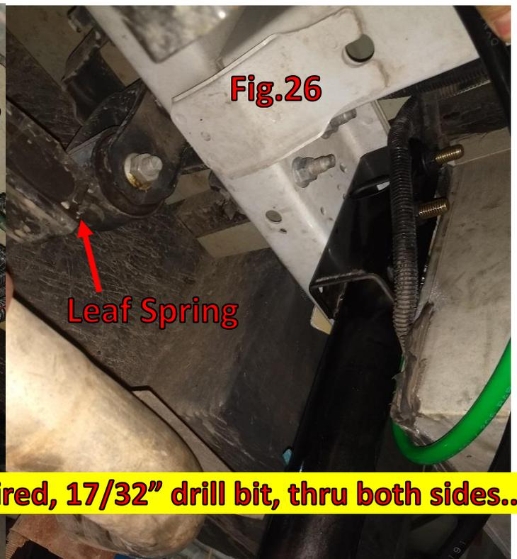
**Using secondary holes, drilling required, 17/32" drill bit, thru both sides..**
