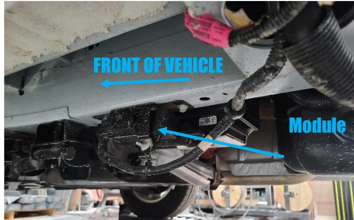
Remove the module with the two M8 self-threading bolts (set aside).
