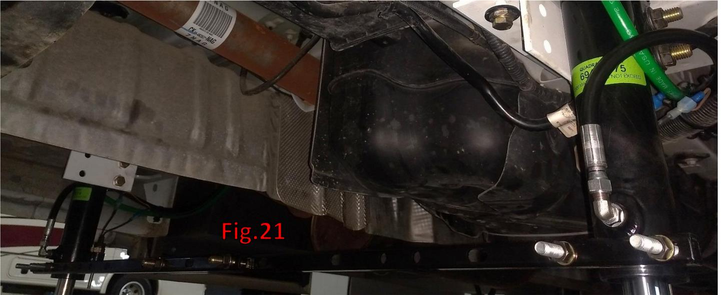
See page 14: ATTACH CROSSBRACE AFTER BOTH JACKS INSTALLED USING 9/16" DEEP SOCKET & WRENCH. SQUARE TUBE & U-BOLTS WRAP UNDER FITTING AND LIMIT SWITCH BARREL JUST ABOVE THE FOOTPAD. FIND TWO HOLES IN CENTER OF UNIVERSAL TUBES THAT LINE UP, INSTALL TWO 3/8" X 2.5" BOLTS, LEAVE ALL HARDWARE LOOSE UNTIL ALL BOLTS ARE IN PLACE, TIGHTEN UNTIL SQUARE BRACE STARTS TO CRUSH.
