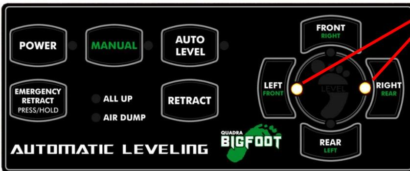
**LEFT FRONT & RIGHT REAR LIGHTS ARE FLASHING, THIS MEANS SYSTEM TIMED OUT, STROKED OUT, OR HAD MOVEMENT DURING AUTO LEVEL. PRESS RETRACT. SEE "TIMED OUT CODE" ON NEXT PAGES.**
