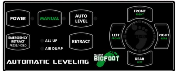
1. Make sure all four cylinders are retracted, if they are move to step 2. If not, turn panel ON, let diagnostic lights flash until they stop (within 30 seconds). Press RETRACT button, when all up light comes, move on.
