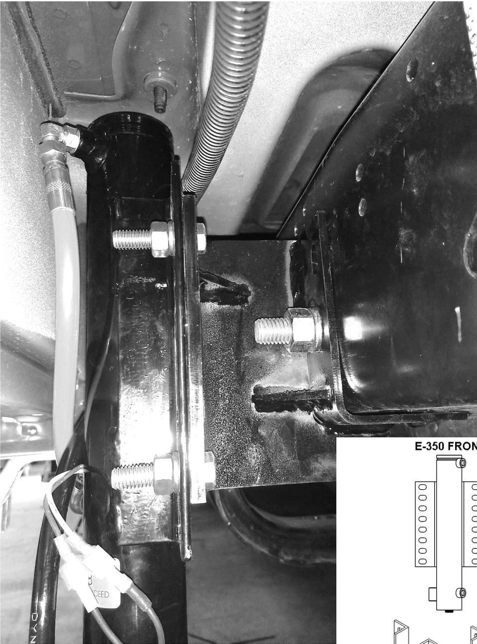
Passenger front shown with 8k13 #M0213F cylinder (perspective facing rear of vehicle). Note how cylinder is mounted above the frame in a "pocket" of the Ford body for higher ground clearance. Fasten cylinder to front mounting bracket with a minimum of four supplied 7/16" Grade-8 bolts 1.75" long with nuts and lockwashers. Make sure cylinder is straight and level, proceed to tighten bolts to 70 ft/lbs.
