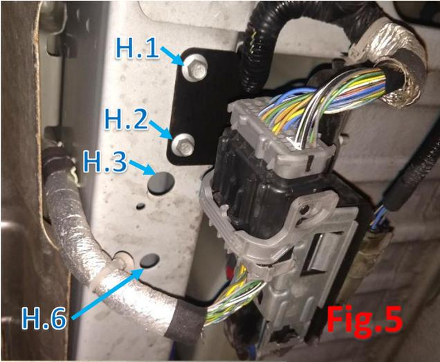
Locate “Front Nox Module” located on passenger front cylinder location under cab’s passenger seat shown in Fig.5. Remove two 8mm bolts with 10mm socket (keep bolts), unclip all plastic rivets releasing the cables from the frame (Fig.6), then slide “mounting tab” from hole in frame as shown in Fig.7, so
