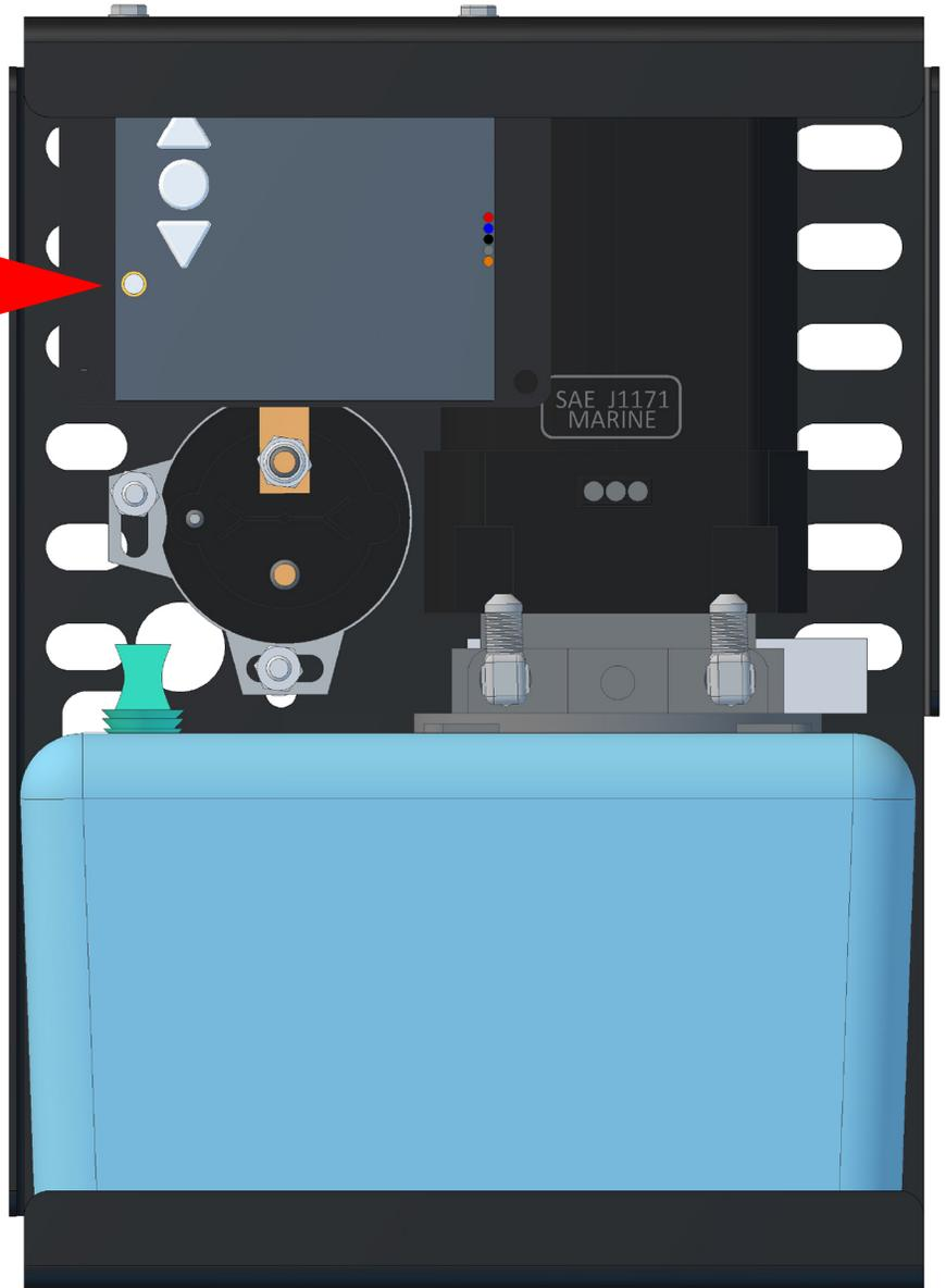
**ATTENTION:** Antenna must be installed in a location outside of the pump assembly.
