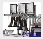
**VERO** camera system for optical print verification. Faulty products will be automatically rejected at the waste gate into a separate box.
