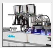
The high precision vacuum transport that handles the products contributes significantly to the excellent print quality and to the highest possible code grading and readability.
