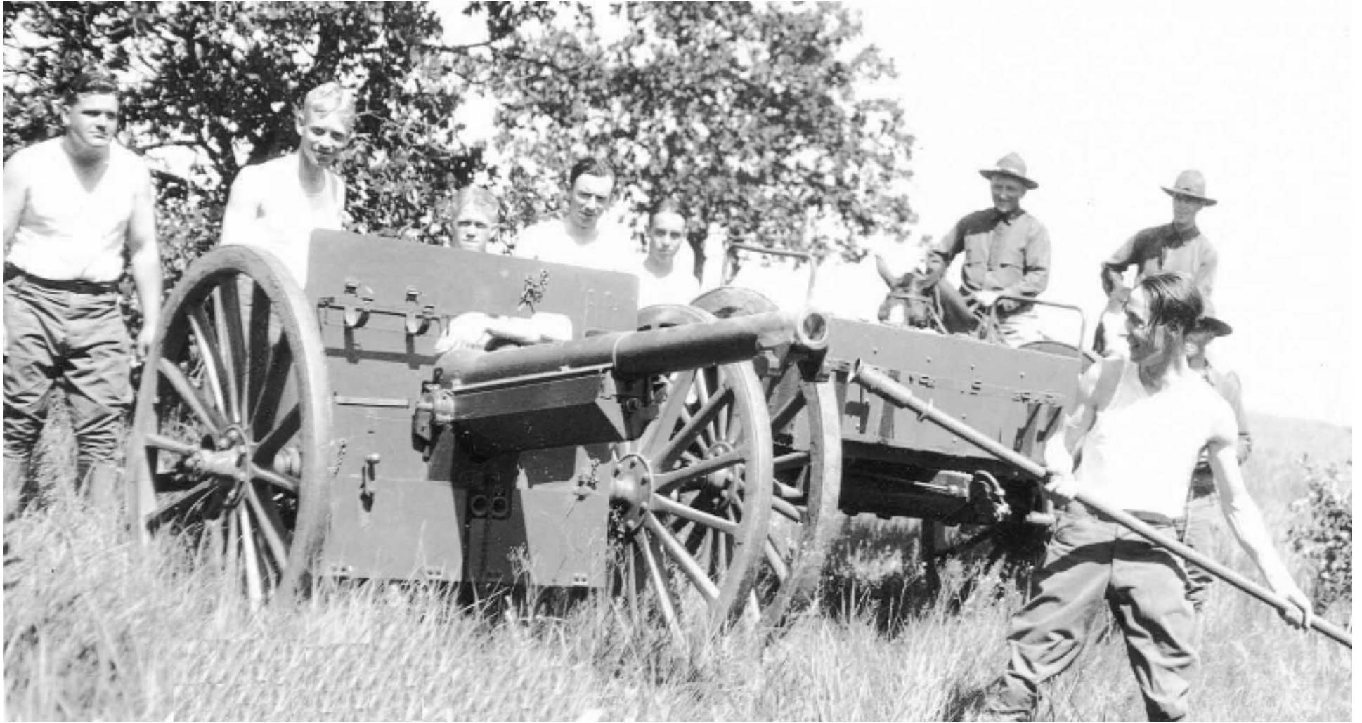
Unit Photograph No. 1: 1927- Battery "C" 158th Field Artillery Regiment-Summer training instruction near Camp Doniphan, Fort Sill, Oklahoma. M1897 75mm gun section and members unidentified. Note the steel tired Archibald patterned spoke wheels indicative of horse drawn artillery. Photograph by Barnard P. Enright of Perry, Oklahoma.
