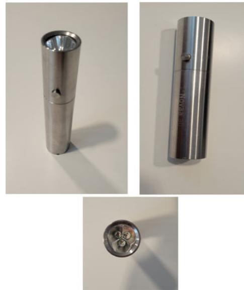
FIG. 1. LED Cluster Head. LED cluster head with red (630 and 660 nm) and near-infrared (850 nm) wavelengths, with an irradiance of 200 \text{ mW/cm}^2 , a beam size of 4.9 \text{ cm}^2 , and a fluence (energy density) of 12 \text{ J/cm}^2 per min, applied for 60 sec over each of the eight, left hemisphere language network target areas during the initial part of a tPBM treatment. LED, light-emitting diode; tPBM, transcranial photobiomodulation.
