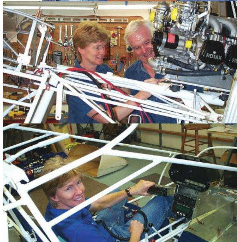
Top: Lisa and husband Jerry. Center: Lisa shows Jerry, then just a friend, how the Rotax 912 installs in a Kolb Mark III in her garage workshop. Bottom: Installing avionics in the center panel of her Kolb Mark III in 2005 in her two-car garage.
