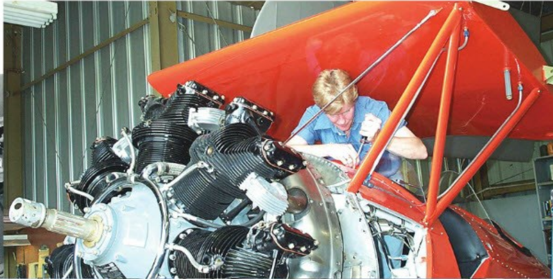
Right: Lisa working on the engine assembly of a 220 Continental installed on a 1931 Waco F-2 in 2004. Below: Lisa rebuilds a bicycle in 1975 as part of her startup business, Turner's Bicycle Service.
