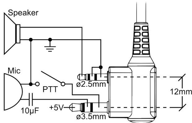
The Kenwood 2-pin connector has one 3.5mm TRS plug, and one 2.5mm TS plug, spaced 12mm apart.
