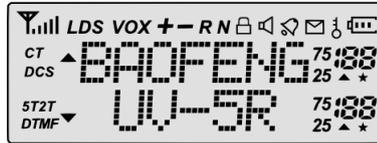
The transceiver is fitted with a seven character by two line dot-matrix alphanumeric LCD, with auxiliary icons for miscellaneous features.
