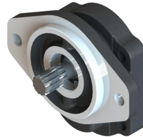
SAE INVOLUTE SPLINE 13 TEETH 16/32 PITCH 13 齿 \text{Ø}21.8 渐开线花键
