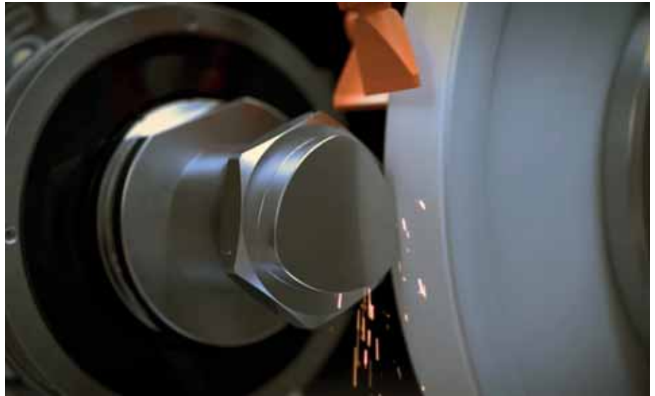
Non-circular grinding of Capto holders.
