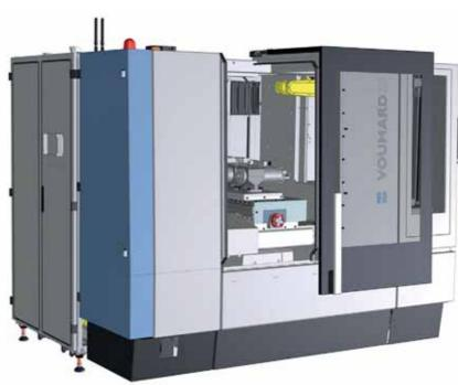
The REX loader automates the VOUMARD 30 without taking up much space. The loading access to the machine room is closed during processing.
