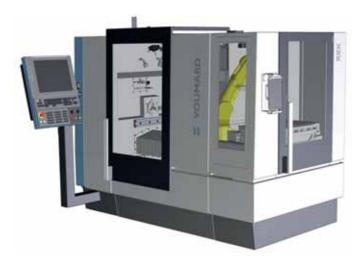
Compact machine, compact automation. The footprint of the of the VOUMARD 30 with robot cell is just  $2.30 \times 1.80$  m.
