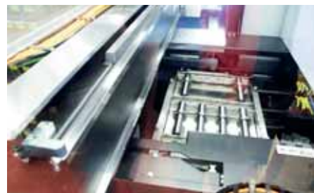
Interior of the WeFlex loader with line gantry and pallet changer.
