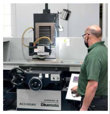
To help avoid the negative effects of heat expansion and vibration, and as an additional support to accurate grinding, the machine's hydraulic unit is isolated from its main structure. A combination of scraped V-V slide ways, the use of low friction Turcite material and the provision of an automatic, gravity-fed lubrication system ensures accurate grinding across the machine's life and results in minimum maintenance needs.
