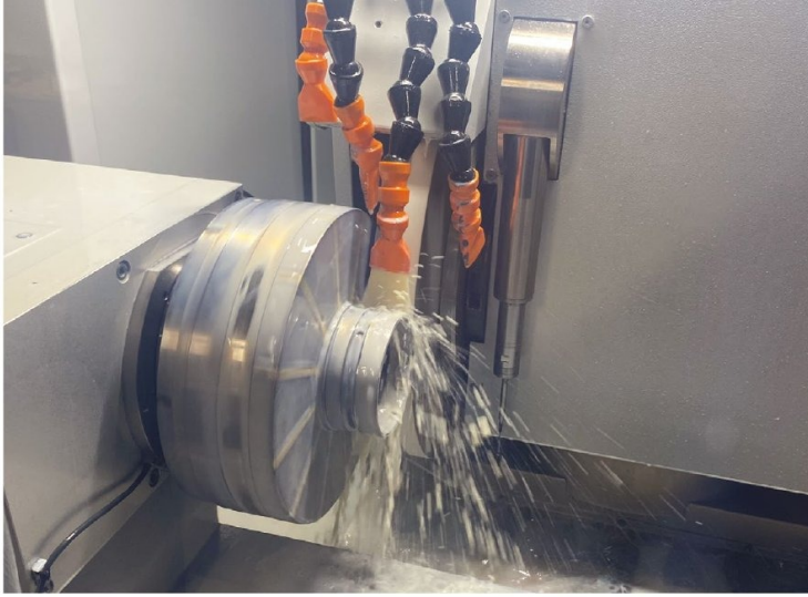
The Wenger WeStep automation system feeding the Kellenberger K100
