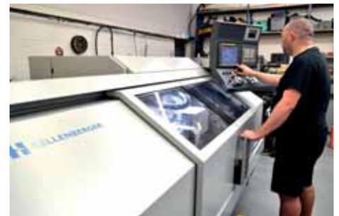
The machine's wheelhead exhibits excellent thermal stability characteristics thanks to the use of optimised spindle bearings and water-cooled motors, in addition the use of thermally-optimised bearings guarantee the highest standards of roundness and dimensional accuracy. To minimise the negative thermal effects of coolant, the machine's coolant tray is separated from the machine bed.
