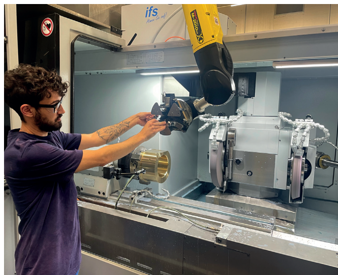
The robot has a three-jaw chuck for the safe transportation of the workpieces. The processing time for this aluminium bronze workpiece is between 45 and 90 minutes
