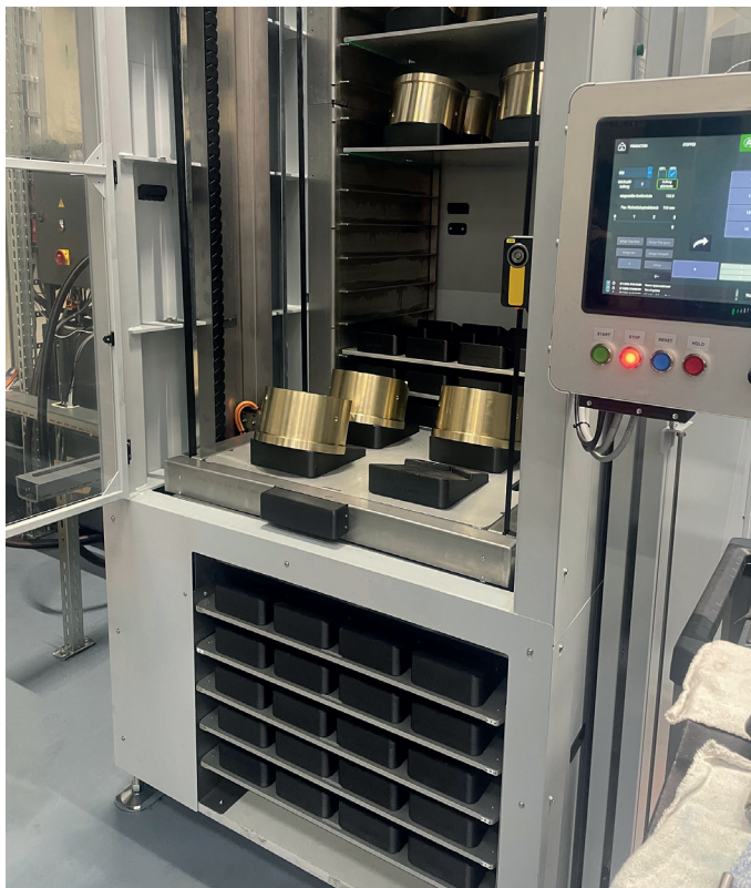
The automated system holds a total of 12 pallets. Depending on the size of the parts, between 36 and 100 workpieces can be set up
