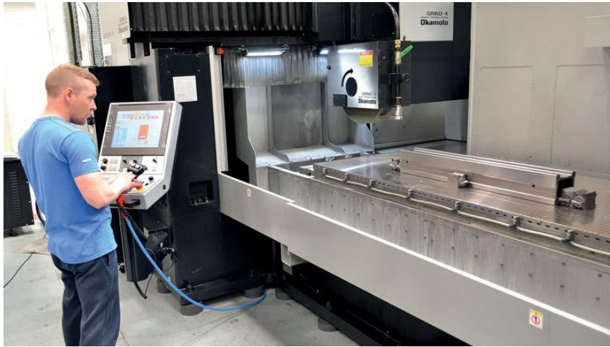
An Okamoto 208 CH-iQ high precision surface grinder recently installed by DF Precision at Ametek Taylor Hobson’s facility in Leicester
