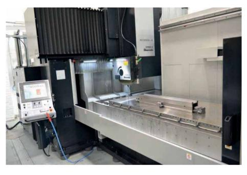
enable the company's components to be ground with outstanding levels surface finish, straightness and form precision. In turn, our ability to grind to the highest of standards of precision helps the company to develop and manufacture ultra-precision metrology products that measure surface finish and form to the very highest standards.
