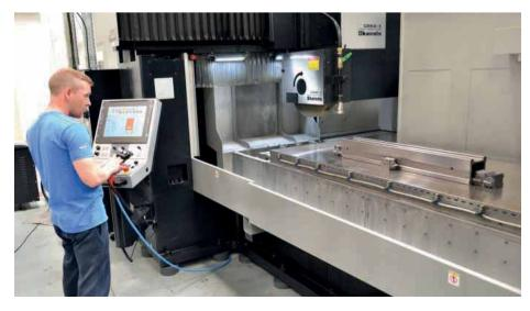
flatness. For example, we now grind our 600 mm long columns to an impressive straightness value of 0.5 µm. In addition to the precision of the Okamoto ACC-CHiQ. the machine's impressive speed is also enabling us to achieve the production efficiency levels we aim for."
