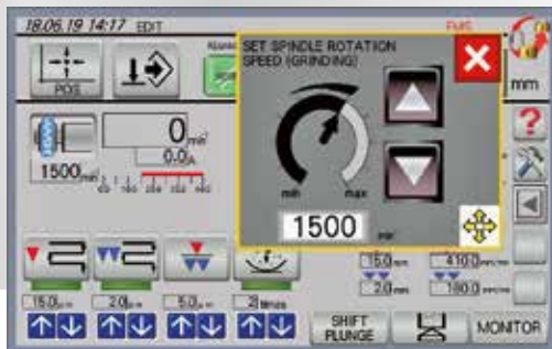
Setting the speed with dial
