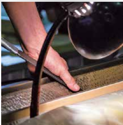
Hand scraped double V table ways
