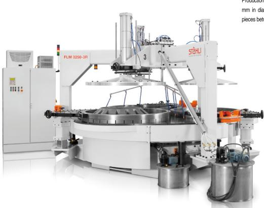
Production lapping machine for parts up to 1500 mm in diameter. Programmable force on work pieces between 0-750 daN.
