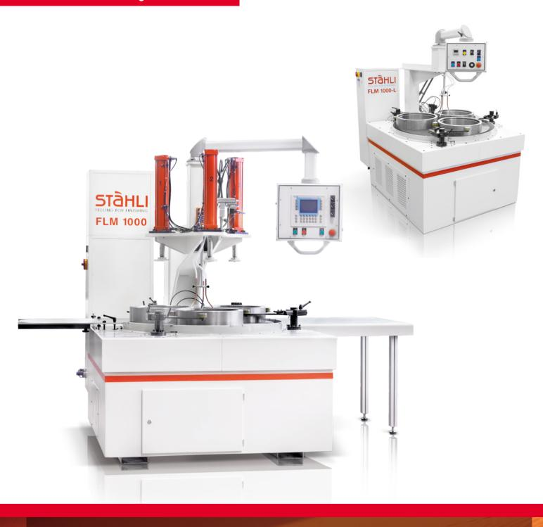
Lapping or polishing with free-rolling particles or flat honing with fixed or super abrasive wheels – the machines of our FLM 750 – 1500 range are real all-rounders. Their employment in both large and small manufacturing shops is multipurpose and includes single piece machining as well as performance oriented series production.
