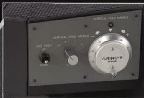
Vertical Feed Manual Pulse Generator Precise vertical positioning of 0.001 - 0.01mm per manual pulse feed.
