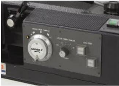
Cross Feed MPG Precise cross feed positioning in increments of 0.0001mm
