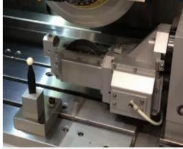
Reference Sphere to be probed before measuring the workpiece
