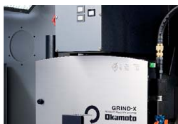
Overhead wheel dresser (with dress compensation)
