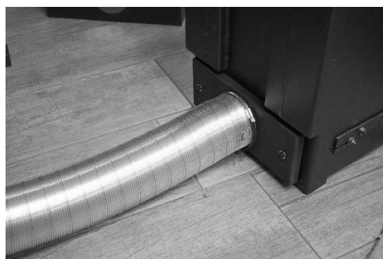
(Image showing direct airbox on Eco 400 version)
