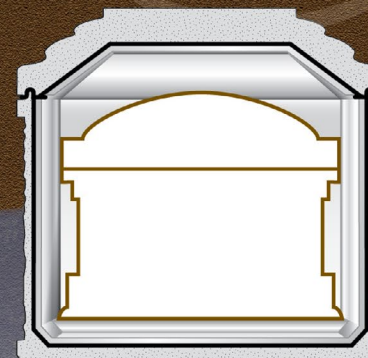
Standard Lined and Sealed Burial Vault
