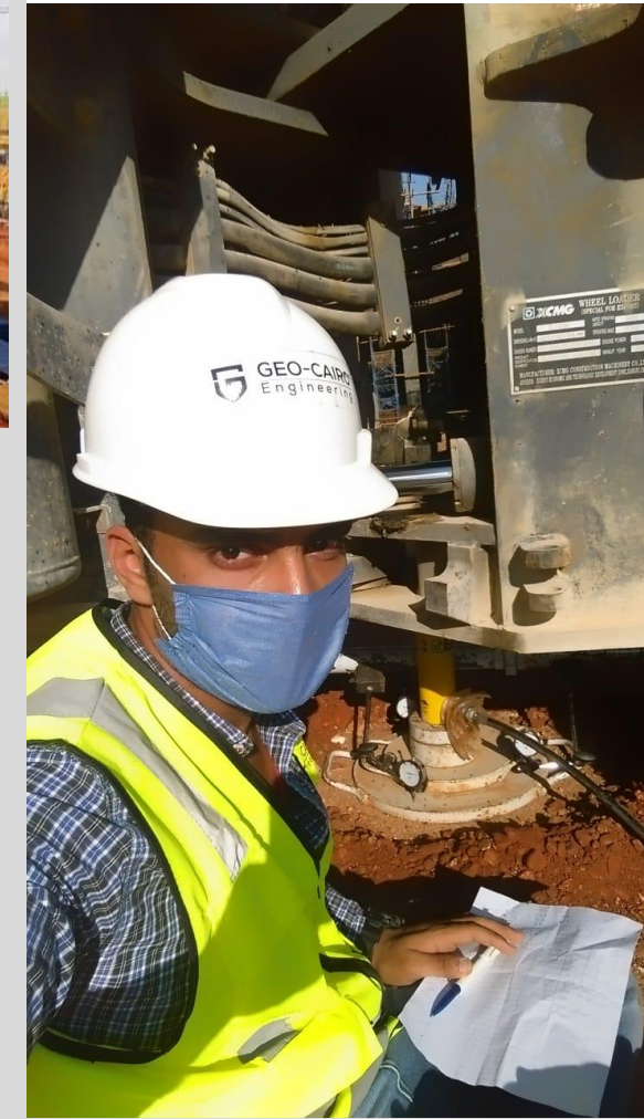
Static Plate Load Test
